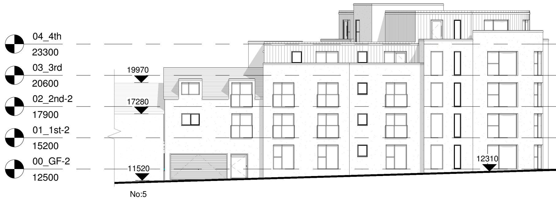
South West Elevation 1 : 200
